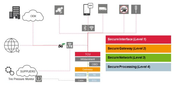
Figure 3: Layered security solution based on automotive levels
