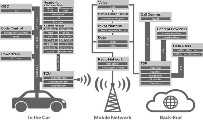
Figure 1: Attack vectors of modern automotive eco-system
